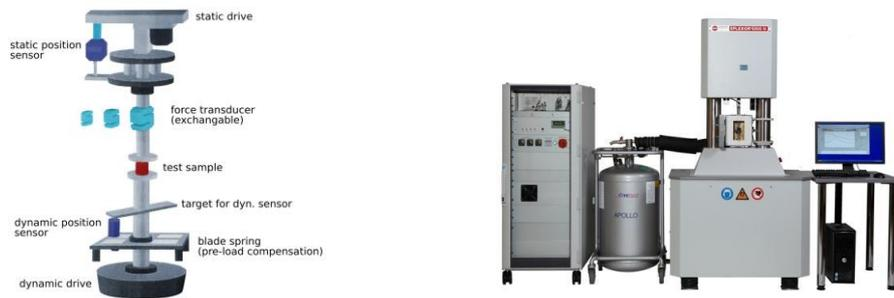
Figure 9: principle of operation of the DMTA (left) and GABO 'EPLEXOR' (right), from [9]
