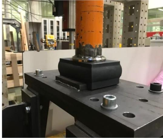
Figure 7: Test setup of the quasi-static and cyclic investigations of sliding bearing and spring
